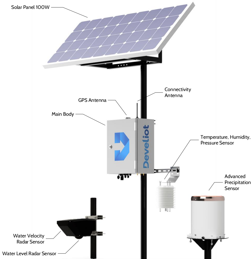
Figure 3: Water Monitoring Station with Water Level Radar Sensor, Water Velocity Radar Sensor, Advanced Precipitation Sensor, and Temperature, Humidity and Pressure Sensor
